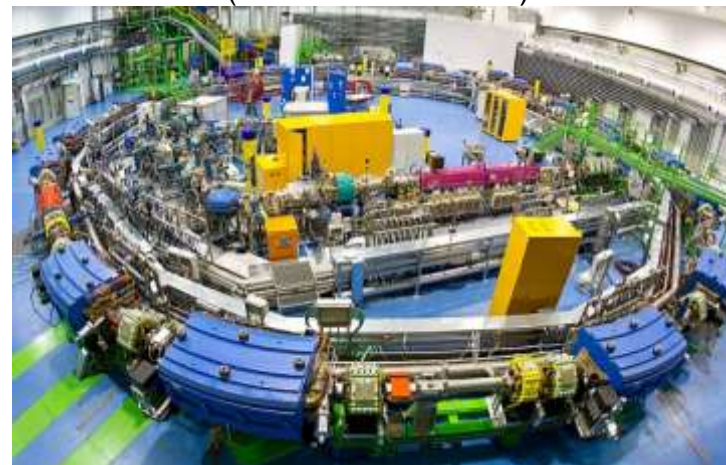
CNAO synchrotron: 78 m long, 25 m diameter (for 400 MeV/u ^{12}\text{C}^{6+} )
